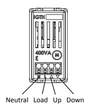
Typical Shutter Wiring Schematic Diagram 2
