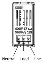
Typical Alternative Switch Wiring Schematic Diagram 2
